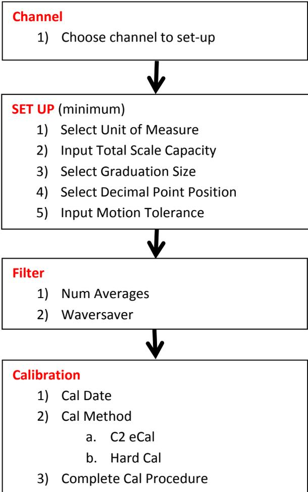
**Calibration:** Section used to calibrate the instrument to the sensor(s) used.
