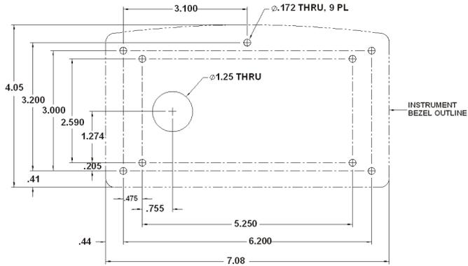
**FIG. 1 PANEL HOLE DIMENSIONS**
