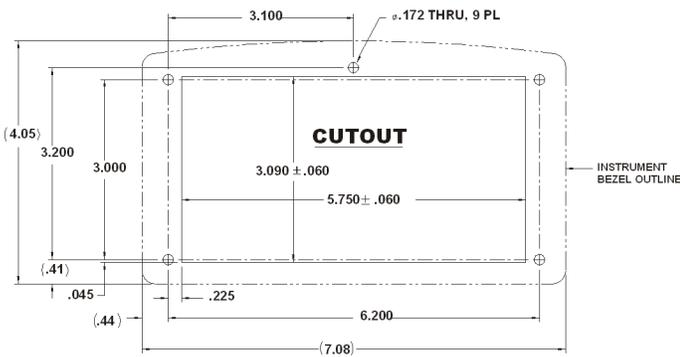
**FIG. 2 PANEL HOLE DIMENSIONS (RETROFIT)**
