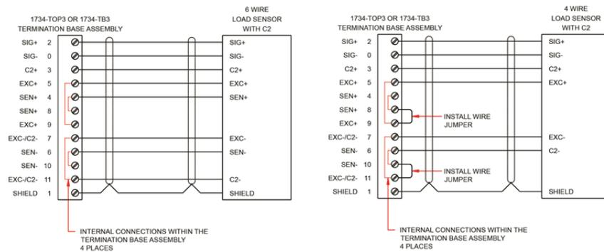
**CAUTION:** Over tightening screw down terminal blocks can shear sensor wires and cause intermittent or complete failure of the weighing system.
