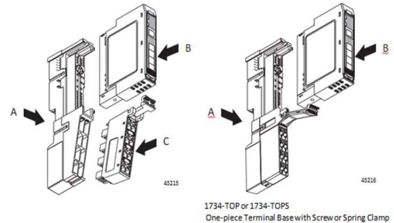
The base (A) mounts onto the DIN rail and provides the backplane. Bases and Terminal blocks are available from Allen Bradley. The HI1734-WS module (B) snaps into the base, **set the KEY position to 2**. The optional removable terminal block (C) also snaps into the base and provides terminations for field-side connections, as well as system power for the backplane.
