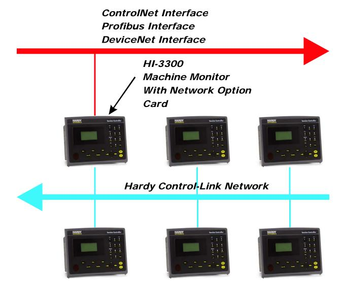
FIG. 6-45 HARDY CONTROL-LINK NETWORK CONNECTED TO A CONTROLNET/DEVICENET/PROFIBUS NETWORK
