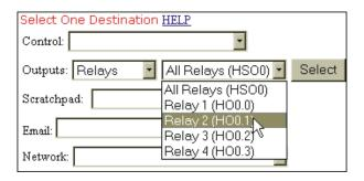
FIG. 6-19 OUTPUT RELAYS/SELECTING RELAY 2 (HO0.1)
