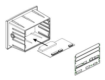
FIG. 3-11 MAIN CONTROLLER BOARD INSTALLATION/LINING UP BOARDS WITH THE SLOTS
