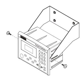
FIG. 3-9 TENSION CONTROLLER INSTALLING IN A SWIVEL WALL MOUNT
