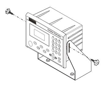
FIG. 3-6 TENSION CONTROLLER INSTALLING IN A SWIVEL MOUNT
