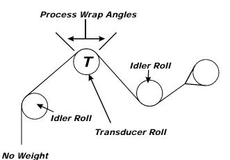
FIG. 5-8 CALIBRATION SETUP WITH NO WEIGHT
