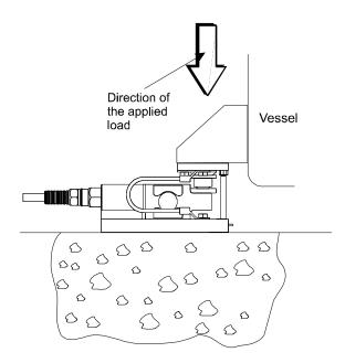
FIG. 5-46 PROPERLY INSTALLED LOAD CELL WITH NO BINDING
