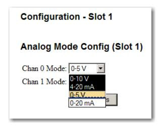
FIG. 4-78 CONFIGURATION SLOT 1/SELECTING CHANNEL MODES
