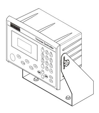
FIG. 3-7 TENSION CONTROLLER INSTALLED IN A SWIVEL MOUNT
