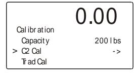
Step 8. Press the Enter button. The C2 CAL Sub-menu appears with the cursor in front of "Load Sensor Num". (See Fig. 5-26)
