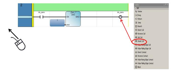
20. Once the ladder rungs are completed, the project will need to be complied to check for any errors and prepare it to be uploaded into the PLC.
