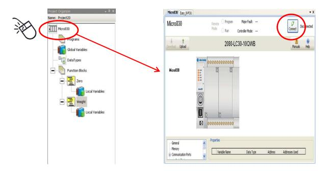
Click on the Connect Button and select the communications path to the processor. In this example the USB port connection was used, click OK.
