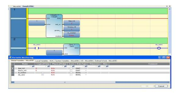
NOTE: If a rung is red then it is in a True state, if it is blue then it is a False state. In the example below the first rung, which is running continuously is red and the second rung, which is conditioned with a trigger bit before it can run is blue.
