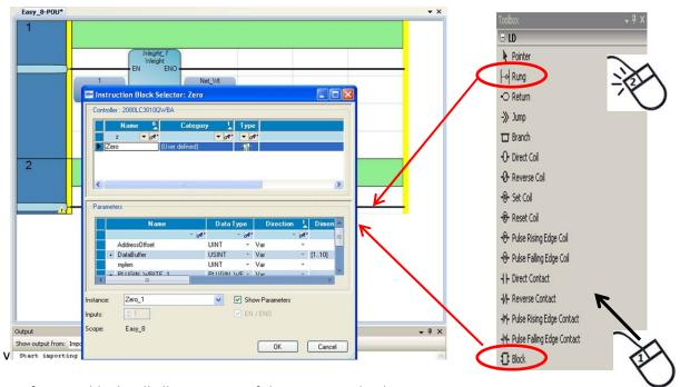
The Zero function block will allow zeroing of the gross weigh when run.
