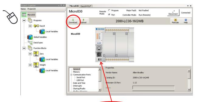
NOTE: Depending on the position of the "RUN-REM-PROG" witch on the PLC, it may necessary move the switch to either the program or the remote position to complete the download.
