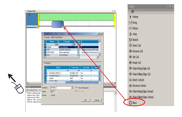
11. From the list by name, scroll down and select the function block to be inserted.
