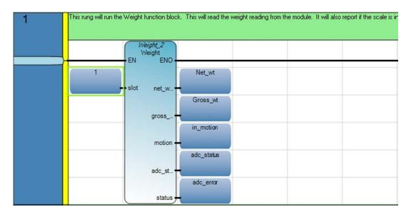
In this example, the weight readings will be continuously updated, no further conditions will be placed on this rung.
