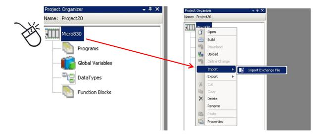
5. Select IMPORT EXCHANGE FILE and navigate to the EASY 8 FUNCTION BLOCK file. (download: http://www.hardyinst.com/process\_weighing/plc+plug-in+modules/easy+8%99+series+weigh+scale+module) Select ALL or just the function blocks required for your project.
