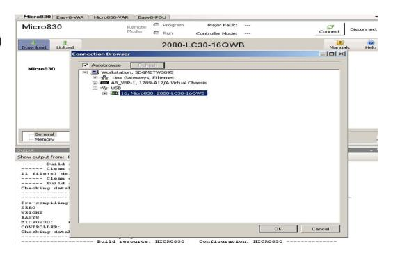
21. Once a connection has been established, download the program to the PLC by clicking on the Download button as shown.
