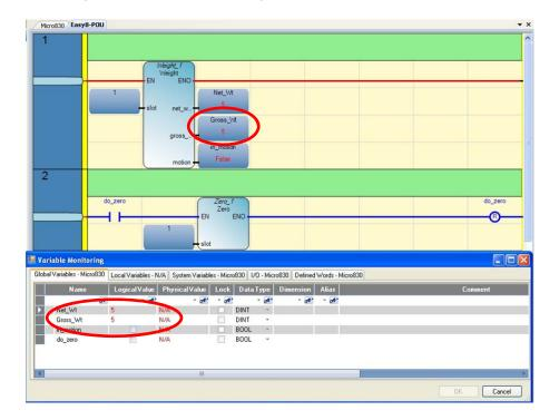
26. In the Variable Monitoring window, click on the box for Do\_zero logical value to change it from low to high. The result of turning on the Do\_zero bit will cause the gross weight to be zero'd. Notice in the example below that the gross weight reading has gone to zero.
