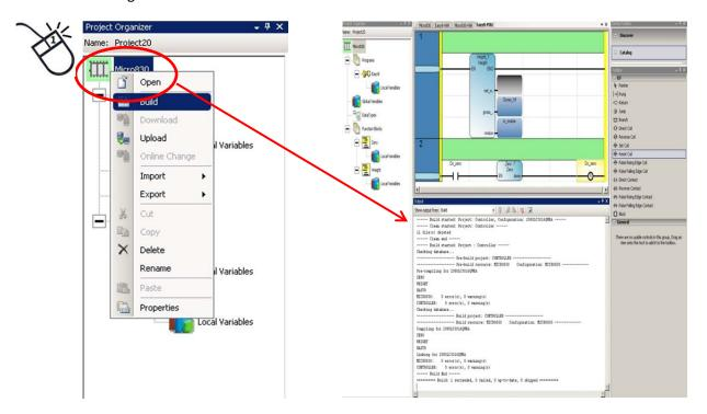
Once the project has gone through the build process, the results will be displayed in the Output window. Here is an example with Output window showing the build was successful.
