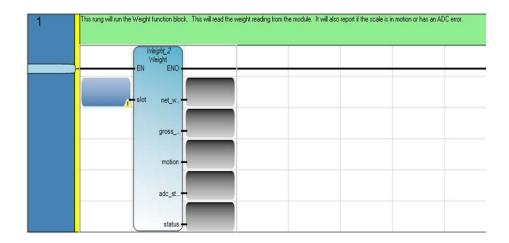
12. The WEIGHT function block has five outputs. A variable must be assigned to each output.
