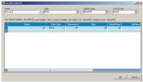
19. To run the Do\_Zero command to only once, the Do\_zero bit will need to be turned off after the function block is run. This is accomplished by using a Reset Coil command from the toolbox. Drag and drop it at the end of the Zero rung and name if Do\_Zero when the variable selector box pops up.
