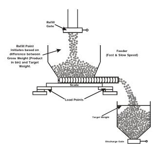
FIG. 1-3 DISPENSING INTO A VESSEL FROM A FEEDER
