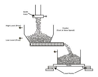
FIG. 1-1 FILLING A VESSEL USING A FEEDER
