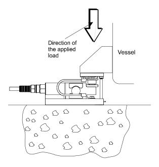
FIG. 2-1 PROPERLY INSTALLED LOAD CELL WITH NO BINDING
