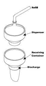
FIG. 5-37 DISCHARGE DIAGRAM
