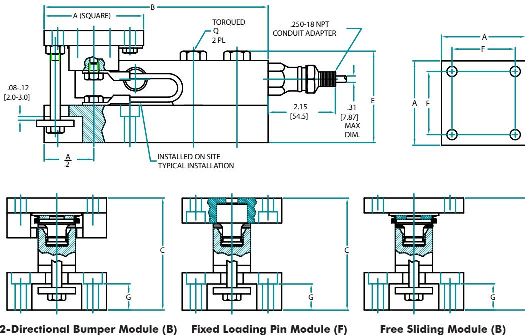
Drawing shown includes HI SBH04 sensor. Substitute Sensor ONLY for HI LPS05 drawing. Other drawings available on Hardy Website
