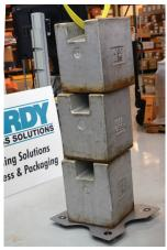
Overload testing was performed on the HIBSX 24 x 24-inch with a capacity of 1300 lbs using three 1,000 lbs test weights. The scale was operational and tested accurate with test weights even after this grueling test.
