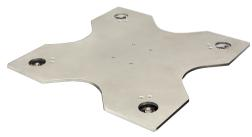
The HIBSX 24 x 24 inch bench scale is designed with an extremely durable all stainless-steel 'X' construction with four planer beam load cells and an integrated HI6011 junction box. With a single platter, this provides an extremely low-profile form factor.
