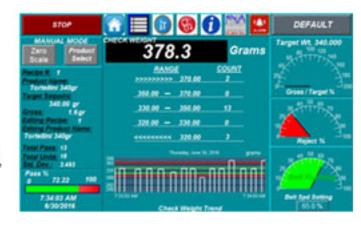
The Dynamic Checkweigher is a fully automated system designed to weigh items in-motion. The Checkweigher controller can communicate both upstream and downstream across the Connected Enterprise.
