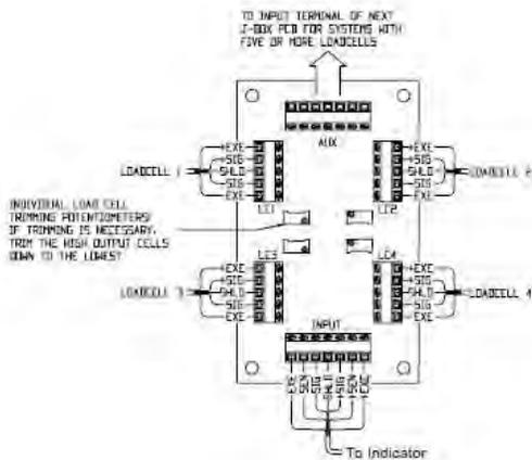
Fig. 6 Hardy 6 Wire C2 Load Cell
