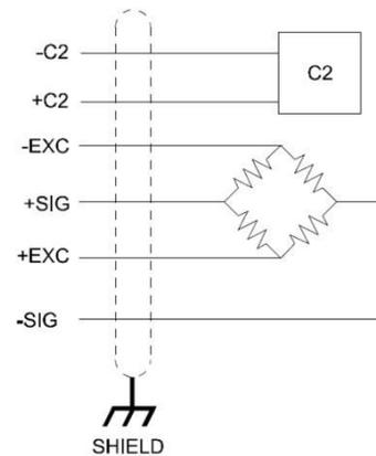
Fig. 8 Hardy Summing Card with C2 and IT (Integrated Technician)
