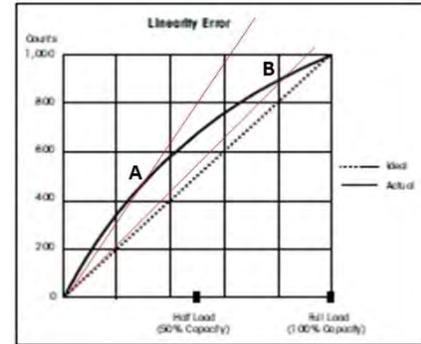
Fig. 4 Linearity Errors
